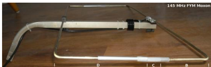
Figure 5. 145 MHz Moxon made from scrap antenna material. Note the RG213 PE-dielectric ('C').
