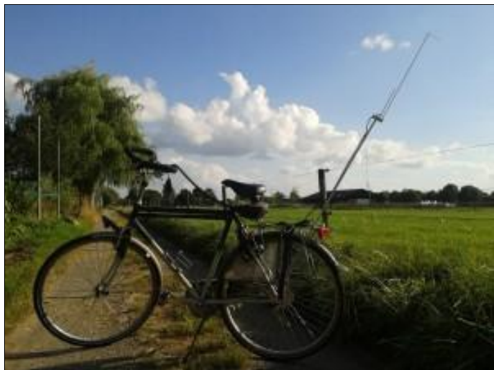
My bicycle with 70cm J-pole antenna attached to the carrier.
